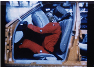
b / The airbag increases \Delta t so as to reduce F = \Delta p / \Delta t .
